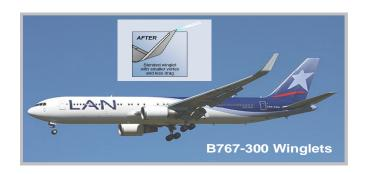
Installation of winglets in all the B767 fleet
